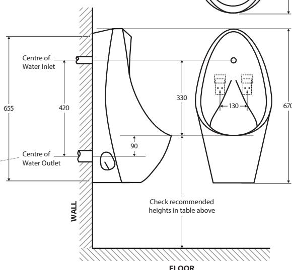
All installations should be carried out by a qualified tradesman in compliance with the National Plumbing & Drainage Code and any State or Local Authority Regulations, in accordance with AS/NZS 3500 series of standards and AS/NZA 6400. All measurements are in millimetres and are subject to change without notice. For ceramic products, please allow +/- 10 mm tolerance for manufacturing variance. Please refer to [fienza.com.au](http://fienza.com.au) for the latest product specification.
