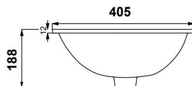
Note: All dimensions are in millimetres and are subject to normal manufacturing variances. Physical Product must be proofed and measurements confirmed before any alteration to installation area is conducted. Studio Bagno reserves the right to alter dimensions at any time. Date created: 22/08/2024
